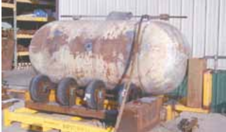
Home-built machine is designed to cut old 500-gal. LP tanks into fire rings, burn barrels, and more.
