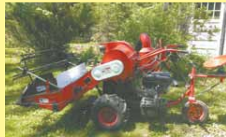
Boaz Mini Combine is designed to harvest grain from small plots. Mini combine has twin cutter bars - one mounted on the gathering reel to clip the grain heads, and the other mounted near ground level for cutting straw.
