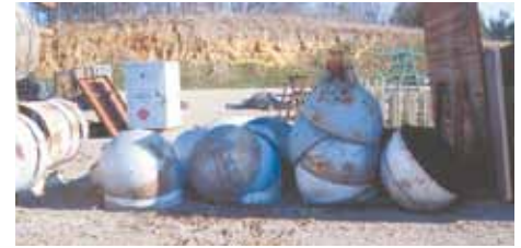
Schley cuts fire rings from 12 to 18 in. high (left). On other tanks he cuts off one end to make boilers, or both ends to make culverts.
