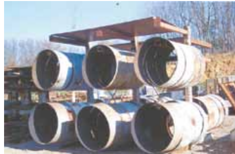
Schley cuts fire rings from 12 to 18 in. high (left). On other tanks he cuts off one end to make boilers, or both ends to make culverts.
