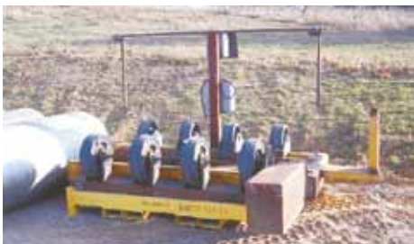
Machine cradles tank on 8 rubber wheels – 4 idlers and 4 drivers – and rolls tank while it's being cut with a plasma cutter that mounts on a metal arm.
