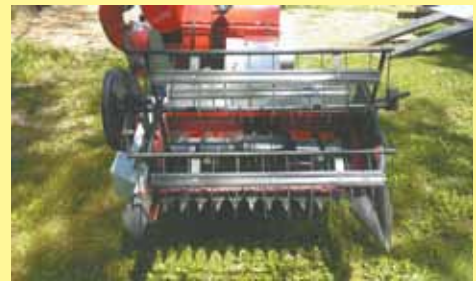
Boaz Mini Combine is designed to harvest grain from small plots. Mini combine has twin cutter bars - one mounted on the gathering reel to clip the grain heads, and the other mounted near ground level for cutting straw.
