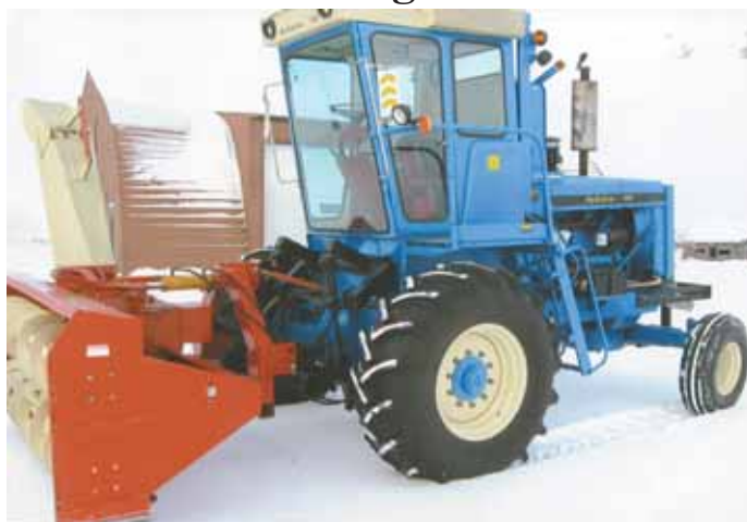
“Nothing comes close to the adaptability of IH 815 and 915 combines,” says Herb Hallman, who converted an 815 model into this utility tractor. He uses the tractor's front-mounted 3-pt. and pto to operate a snowblower.
