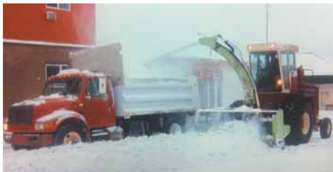
Kevin Ford converted a Case IH 915 combine into a tractor that he uses to blow snow into trucks.
