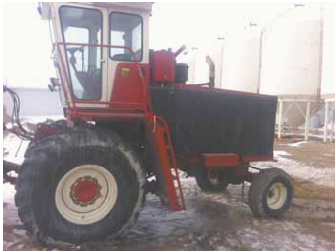
After stripping down the combine, Ford repositioned the components he needed on an old truck frame cut down to 14 ft.
