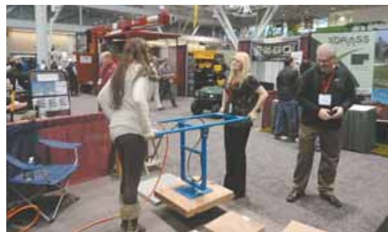
Paver Placer uses an air compressor to create vacuum to lift and place heavy stones.
