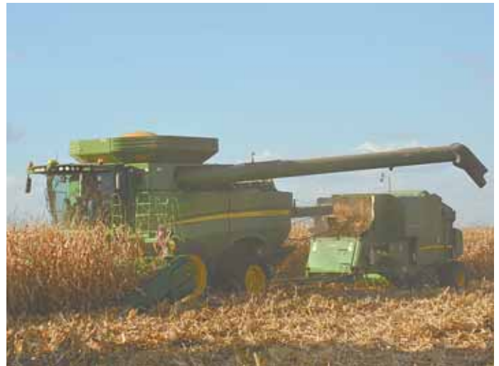
Deere's Single Pass Round Bale system attaches to the back of Deere S670, S680 and S690 combines equipped with ProDrive transmissions.
