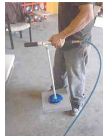
A Venturi trigger on handle provides a quick release of stone.
