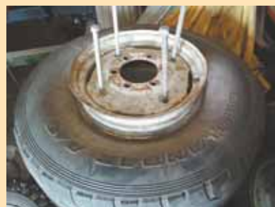
Four long threaded bolts run through holes in the car wheel rim to tie all 3 wheel rims together.
