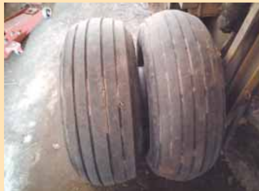
To improve the flotation on his round baler, Arlo Greenberg bought another pair of 15-in. flotation tires, then fitted a 13-in. car wheel rim between each set of tires.
