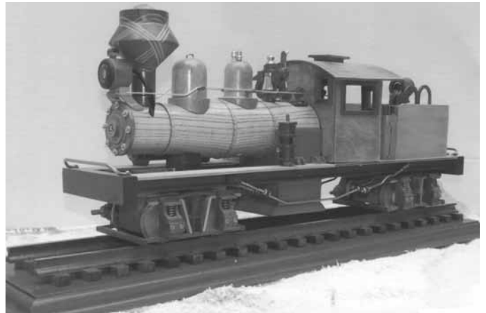
Joe Rishel built this 22-in. long wooden replica of a Shay 2-truck, 28-ton Class B narrow gauge engine locomotive.
