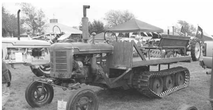
Farmall Super A’s rear wheels were removed and replaced with rubber-coated sprockets, which drive twin metal tracks that are 16 in. wide and 8 ft. long.
