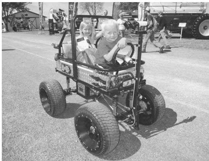
Allen Riegle pulled his 2 kids in this sporty wagon at a recent show. It’s complete with a roll cage, LED headlights, turn signals, a horn, and a waterproof sound system that hooks up to Riegle’s cell phone. The go-kart steering wheel on front is just for looks.
