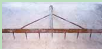
Miller uses his Cub Cadet garden tractor to pull this 6-ft. wide "bottom rake" across bottom of pond.
