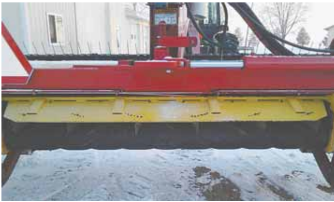
Photo shows "wide switch" kit that mounts on back of haybine. Six 15-in. long fins deflect hay out to both sides.
