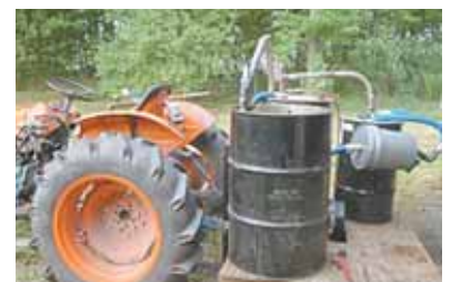
Home-built gasifier chemically transforms grass pellets into a form of hydrocarbon fuel that powers Dave Dolan’s small diesel tractor.
