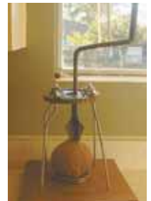
Place coconut on metal ring inside stand, then turn handle fitted with blade to remove shell.
