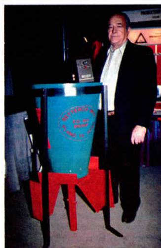
New electronic spreader can be used on any size bin - up to 60 ft. dia. - without any change in hardware.
