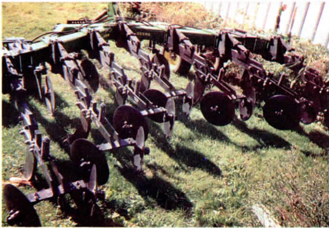
A pair of disc levelers mounts behind each shank, mounted on a bracket that bolts directly to the V-ripper shank.
