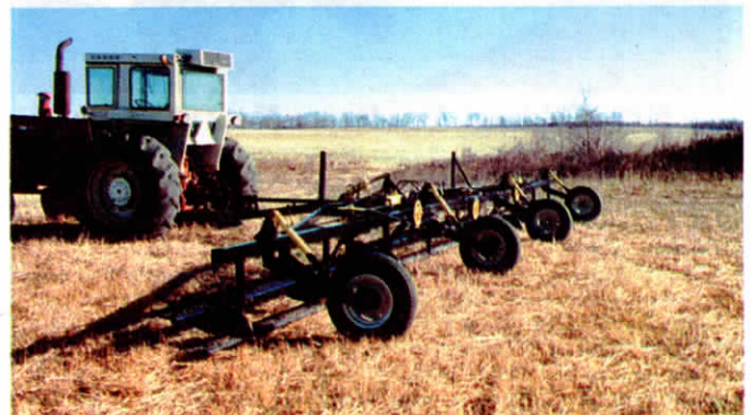
The belt-driven, pto-powered double cutterbar lets farmers cut crops higher off the ground when harvesting to improve efficiency of combine. A trip is made through field later to cut straw.
