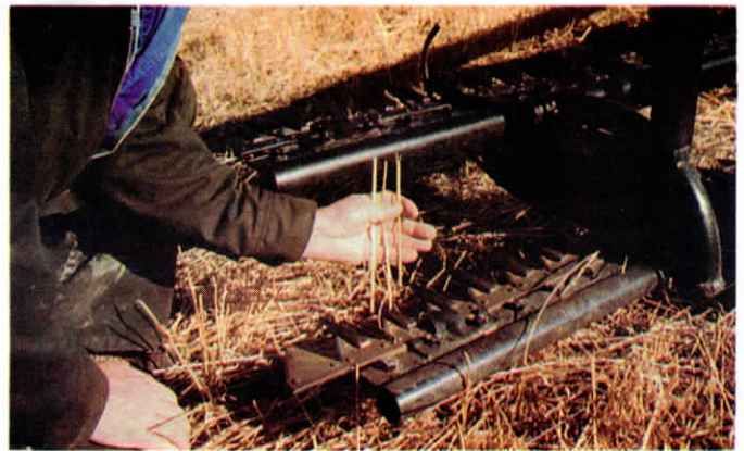
There’s 8 in. between the top and bottom cutterbar, and the top cutterbar is positioned 8 in. ahead of the bottom bar.
