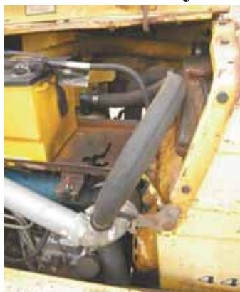
All it took was a little creative plumbing for David Luttrell to fix the “blowby” problem on his 1975 Ford 4400 industrial diesel engine.
