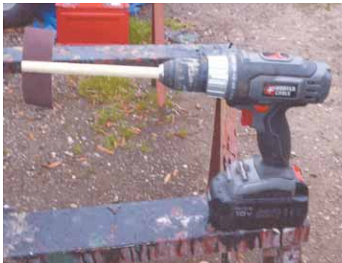
Sanding attachment consists of an 8-in. long, 1/2-in. dia. wooden dowel rod that fits into the chuck on Wallrath’s cordless drill.
