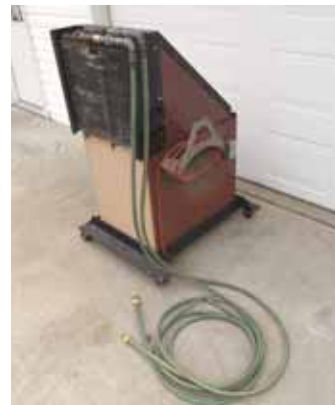
Gary Eberspacher converted an old furnace into this evaporative “swamp cooler” that hooks up to a garden hose.
