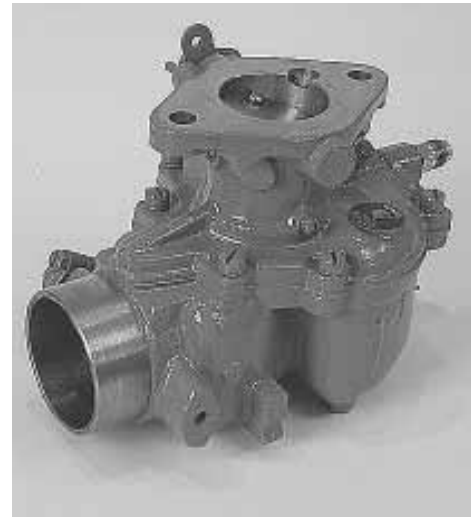
Gary Hoefling says his modified Zenith carburetor cleans up the black smoke and fouled spark plugs common to Deere 3010/3020 and 4010/4020 tractors.
