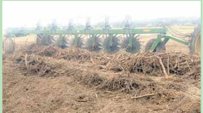
Rock 'n Root Rake has heavy steel fingers that dig down to a depth of about 12 in., pulling out roots and rolling them into windrows.
