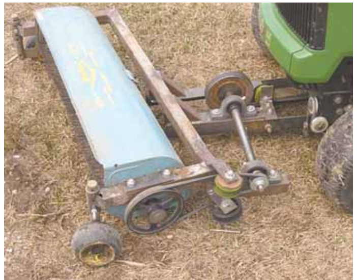
Tom Feuerstein turned an old 32-in. wide, walk-behind sweeper into a power broom that mounts on front of his Deere riding mower.
