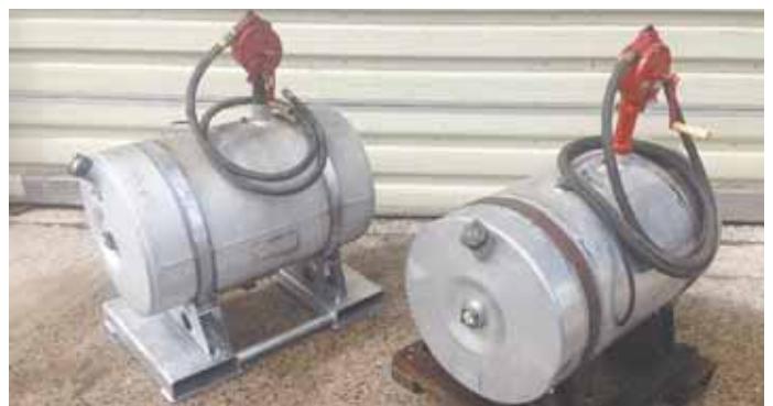
Looking for a simple way to refuel his farm equipment in the field, Leroy Keens converted a pair of 50-gal. aluminum diesel fuel tanks out of semi-refrigerator trailers.
