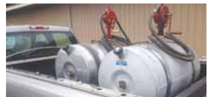
He made mounting brackets for forklift spears. He also welded a fitting on top of the tanks for a hand-cranked pump equipped with a 15-ft. hose.
