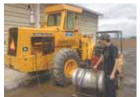
He made mounting brackets for forklift spears. He also welded a fitting on top of the tanks for a hand-cranked pump equipped with a 15-ft. hose.
