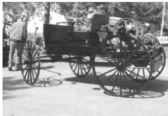
George Feltz converted an old 2-seater horse-drawn buggy into a self-propelled rig, by installing an old Deere hit and miss engine on back.
