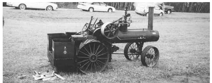
Clarence Hoffman built this 1/3-scale steam tractor. He custom-ordered the boiler but made everything else, with many parts coming from other tractors.
