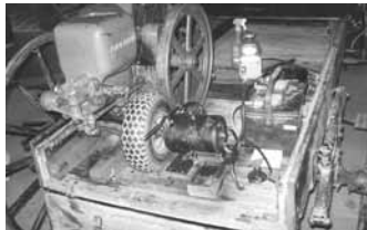
An old Ford Model A car starter wired to a car battery is used to start the engine.
