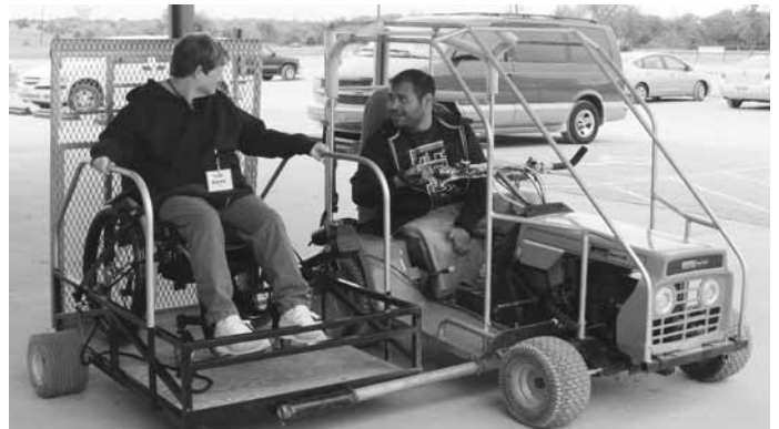
Garden tractors are fitted with sidecars to carry wheelchairs. Tractor controls are modified so disabled drivers can operate them.
