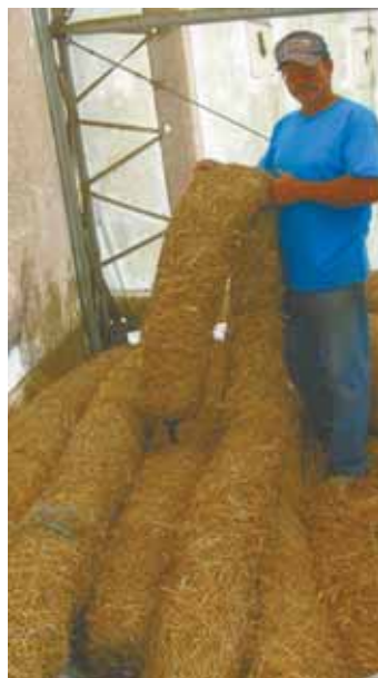
Large straw sausage is held in place by wooden stakes and acts like a mini-terrace on bare slopes.
