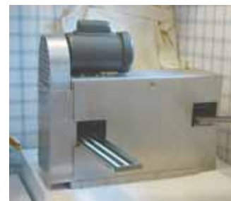
Powered egg washer uses water and a rotating brush to scrub eggs as they pass through machine.
