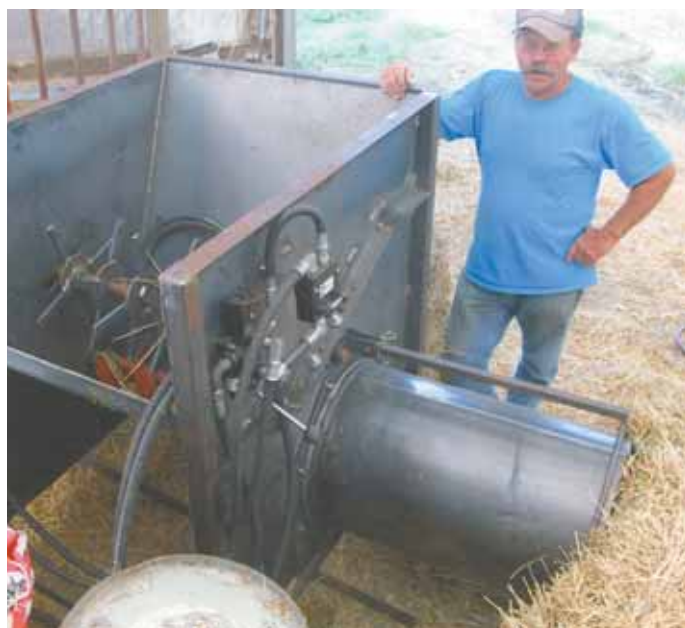
Tim Gogerty built this machine to pack straw into erosion control "waddles".
