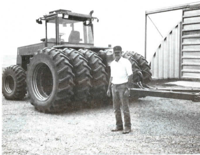
Big Butch's cab sets above and forward of rear tires, providing a panoramic view to all sides. The frame is just 12 in. wide at the rear so the two inside rear tires can be positioned just 24 in. apart.
