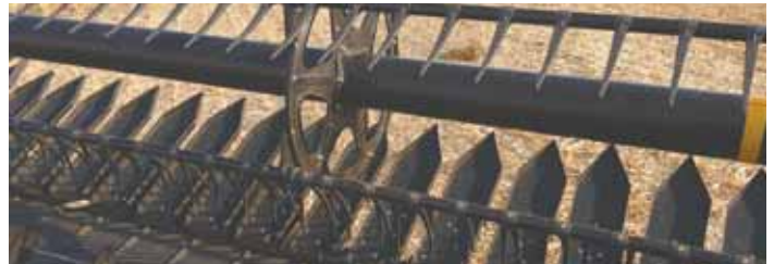
Pans are just over 9 in. wide at the cutterbar and about 3 ft. long. They guide stalks into the cutter bar and make sure ears and the cut stalk move into the auger or onto the canvas.
