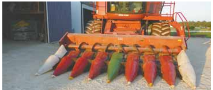
Ross Bishop's home-built IH cornhead contains parts from three International 38-in., 4-row cornheads. He hopes it will run faster than the old head on his International 2166 combine.
