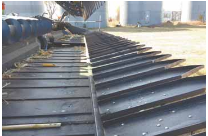
Flexxifinger Corn Harvest Pans let wheat and small grain farmers harvest corn without buying an expensive cornhead. They pop off in minutes to switch back to small grains.
