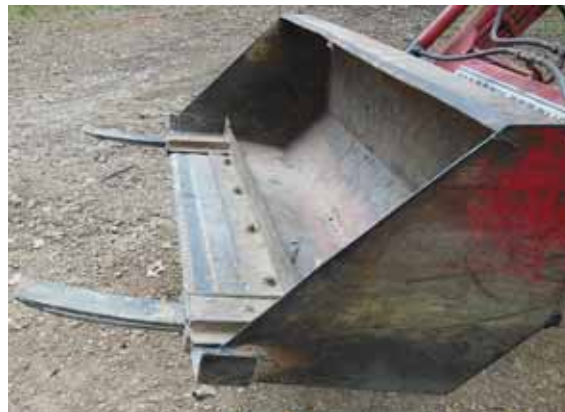
Granville Yates used leaf springs from old trucks to make inexpensive, loader-mounted forks. Each fork consists of 2 springs sandwiched together.
