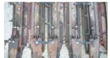
He bought new Calmer 20-in. header snouts and then remounted his existing 30-in. row units.
