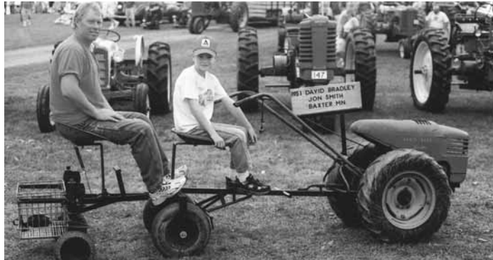
Lonnie Smith used steel tubing to build a pair of 2-wheeled "sully trailers" that are pulled by a 1951 David Bradley walk-behind cultivator.
