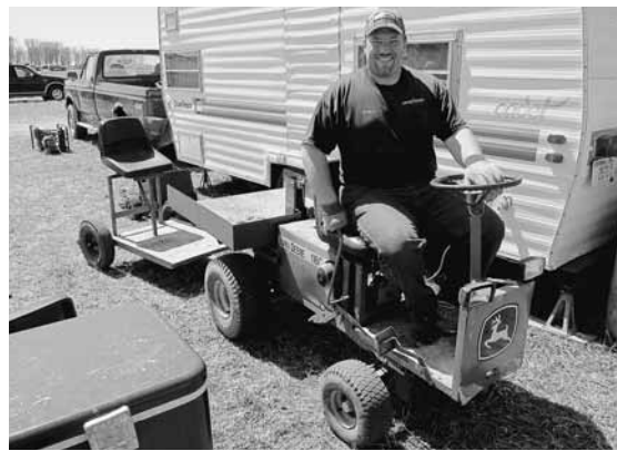
Converted Deere 116 garden tractor sports a dump-style rock hauler on back. A 2-wheeled trailer with a seat mounted on it pulls behind the tractor.
