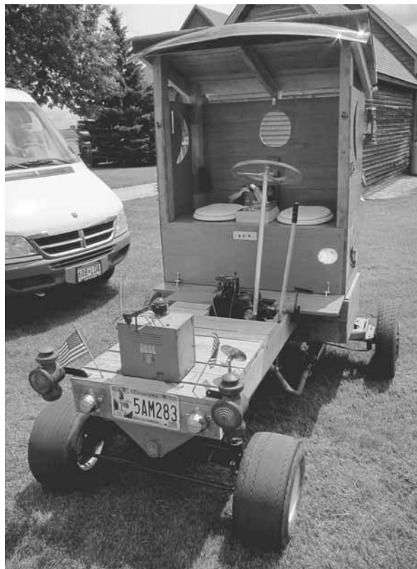
The rider sits on one of 2 cushioned toilet seats fastened to a wooden bench. On front are 3 different "ooga" horns, a siren, an old-time tractor radio, and model T headlights.
