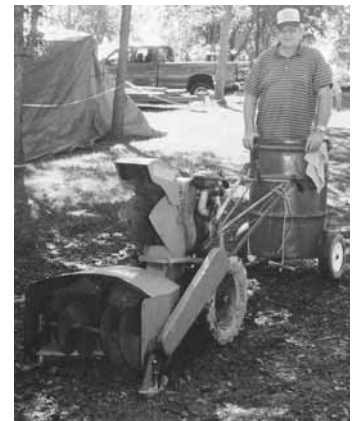
Bob Scheffer built this 2-wheeled "chariot" to pull behind an old walk-behind snowblower.
