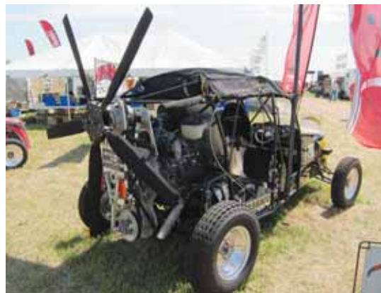
Maverick LSA "Flying Car" is a dune buggy-like vehicle that flies by way of a propeller at the rear and a parachute for lift.
