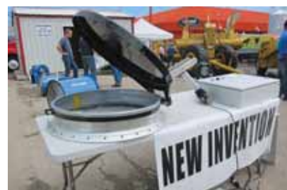
Actuator arm opens bin and also applies up to 200 lbs. of force to keep lid tightly sealed when closed.
