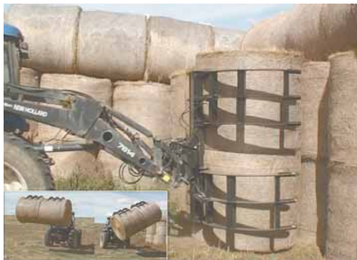
Grapple can grab 2 bales at a time and rotates them 90 degrees.
