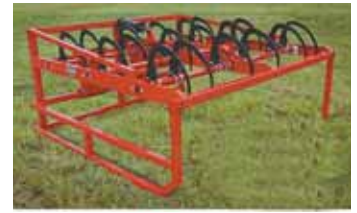
The MEGAGrapple is designed to gather and lift three 8-ft. square bales at a time in either direction. It lifts over the top to easily set hay on a trailer or stack.
