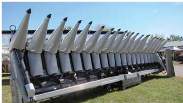
The Tango corn header is made mostly from aluminum, which reduces header's weight by 25 to 40 percent – a big advantage as combine headers keep getting bigger.
