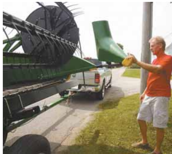
Crop divider hinge attaches to header beam with a welding kit or bolts in place.
