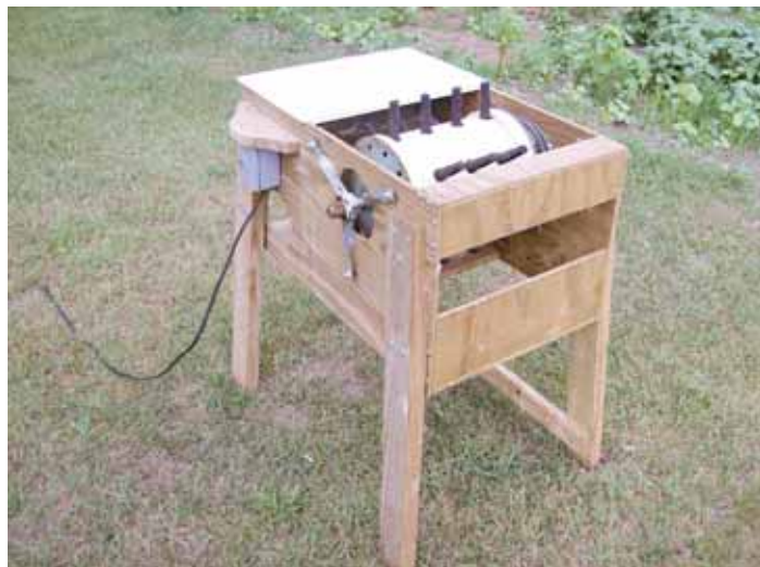
Jack McGee made this chicken plucker out of treated plywood, 12-in. pvc pipe, and parts from disassembled squirrel cage blowers.
