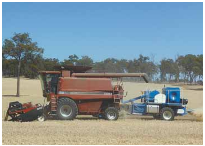
Harrington Seed Destructor destroys weed seeds behind a combine. After a full year of testing across southern Australia, it's now in production.
