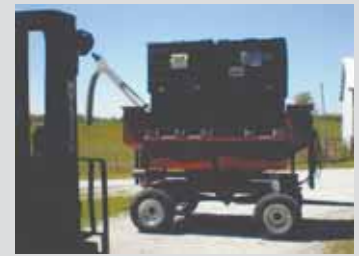
Lester Graber modified a 150-bu. Parker gravity box to carry 2 bulk seed boxes placed side by side. A center divider keeps the seed separate.
