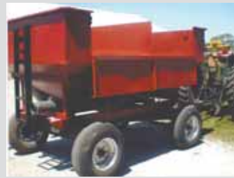
Lester Graber modified a 150-bu. Parker gravity box to carry 2 bulk seed boxes placed side by side. A center divider keeps the seed separate.
