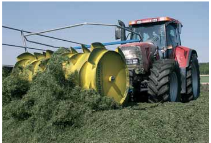
"It throws silage out in front of you and leaves a nice, even layer that results in a tighter silage pile with less spoilage," says Agromatic about its pto-driven Reck silage spreader.
