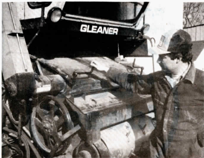
To adjust cylinder clearance, loosen 2 bolts and turn hand cranks.
