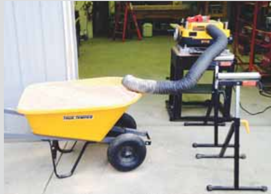
John Houston uses a wood planer equipped with a built-in chip blower inside his shop. He hooked up a plastic hose to a port on the planer and ran the hose into a wheelbarrow covered with landscape fabric.
