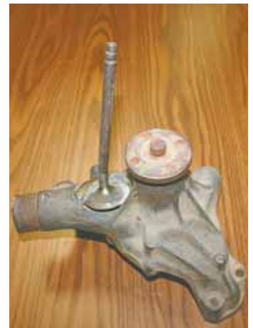
Magna 777 rod provides machinable welds that won't crack on most types of cast iron. Photo shows a steel valve welded to a cast iron pump.
