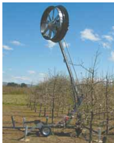
Super-sized portable fan has a 3-bladed impeller that operates inside a shrouded 7-ft. dia. fan head. It can be raised up to 28 ft. in the air on a hydraulic arm.
