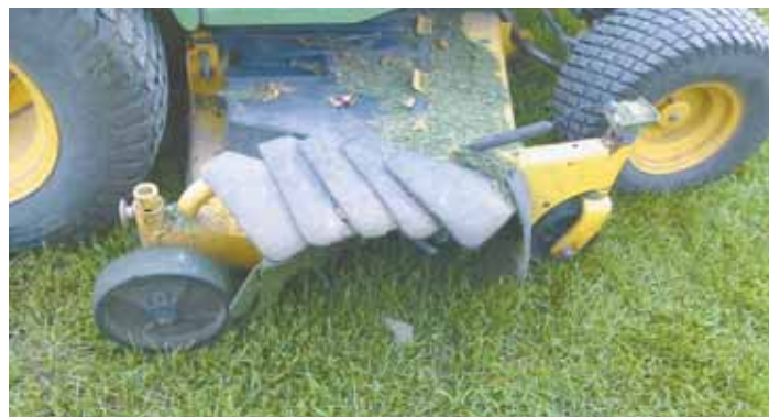
A set of overlapping rubber "ear corn savers" off an old cornhead bolt individually to mower deck, allowing Phillips to adjust flaps individually.
