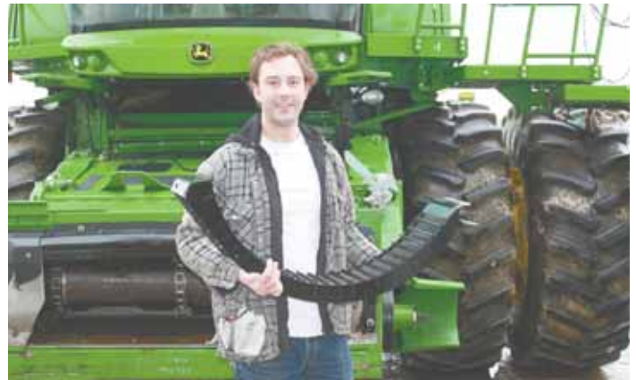
High-wear concaves are fabricated from armor plate grade steel. "It's twice as hard and 4 times as strong as steel in ordinary concaves, so it can handle rocks and sand," says Russ Wildfong.
