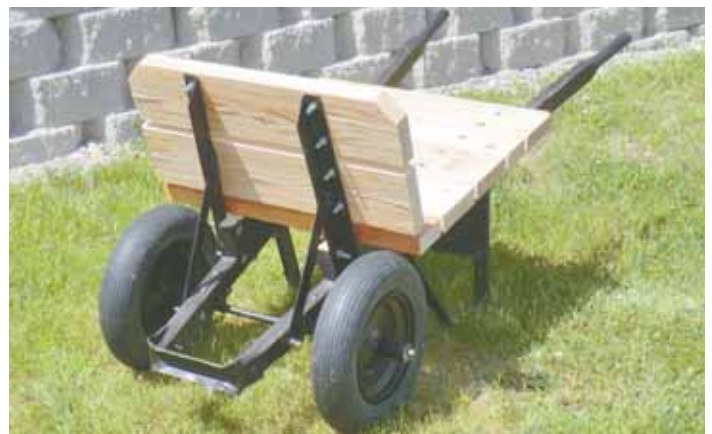
Ray Young converted his 2-wheeled wheelbarrow with poly tub into this wooden "flatbed" that'll handle tougher hauling jobs.
