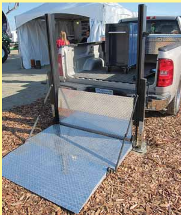
Electric-powered "lift gate" attaches to pickup's receiver hitch to load or unload up to 1,000 lbs. by pressing a button.
