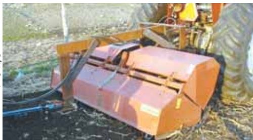
Bridge hitch "leapfrogs" over top of rototiller and bolts to grain drill's tongue.
