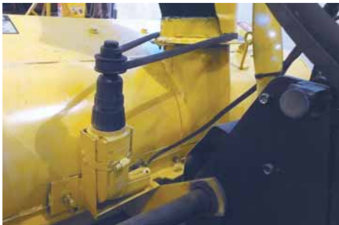
Larry Wood powered the chute on his front-mount snowblower using an old 12-volt cordless drill that mounts vertically in a bracket on back of blower.
