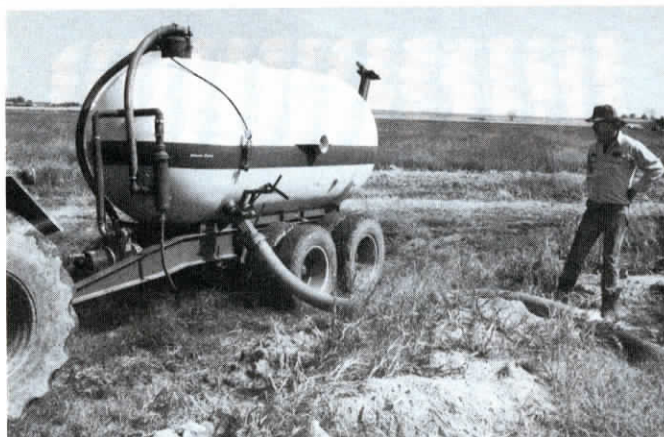
The Johnstons made their spreader out of an old propane tank. To fill, a hose is hooked up to inlet port on lower left side of tank. Note air vane pump on tongue of trailer.
