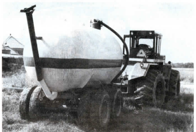
Manure blasts out of tank against hinged plate and is spread in 40-ft. wide pattern.
