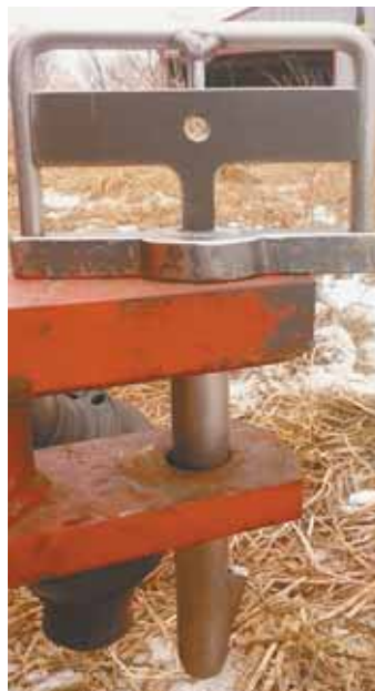
Squeezing the Keep-In-Hitch's handle causes a key at bottom to retract. There's no pin clip that can accidentally get pulled out.
