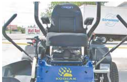
ZTR Puffer air-ride seat can be used on everything from lawn tractors to zero-turn riding mowers and even small compact tractors.
