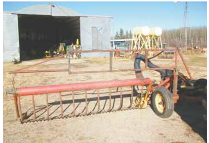
To mount the air reel, he fabricated a support using the boom off an old crop sprayer. "If the boom hits a solid object, it's designed to break away," says Rogers.
