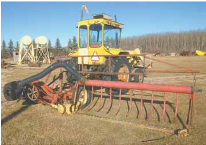
To keep the cutterbar clean on his New Holland mower, Dale Rogers modified the air reel from an old combine and then added a blower off a Gleaner sidehill combine.
