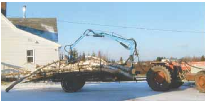
Caissie uses tractor hydraulics to operate this home-built, trailer-mounted log loader. The 20-ft. long rig is equipped with a jib that swivels 180 degrees and also up or down.
