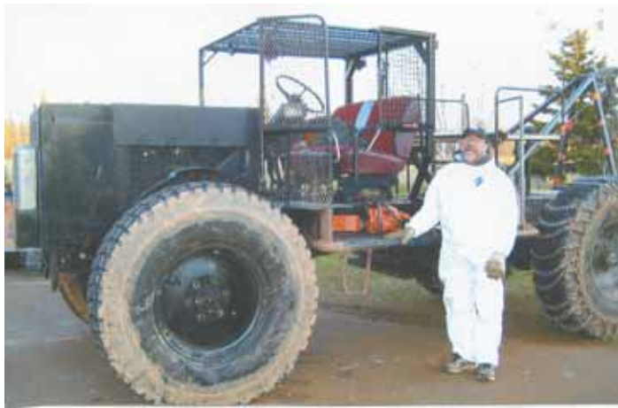
“The big wheels provide a lot of clearance in the woods,” says Alfred Caissie, who converted a 1961 Dodge 3-ton, 4-WD truck into this heavy duty, 4-WD log loader.
