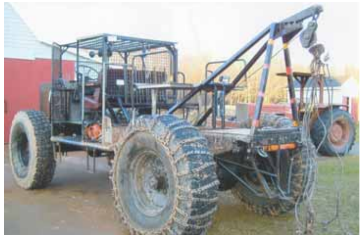
The “Big Rig” has an electric winch on back and 8 chokers attached to a main cable, allowing Caissie to hook onto felled trees and winch them up to the rig.
