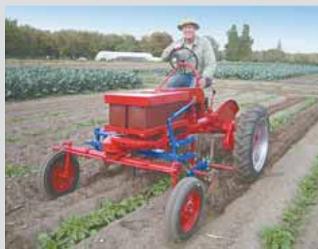
Farmall Cub tractor is powered by a DC motor that hums effortlessly, powered by 4 Trojan deep cycle, 12-volt batteries.
