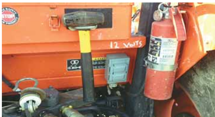
Waterproof, 12-volt AC metal outlet box on back of tractor is wired to tractor's battery. "It eliminates the need for a battery to operate the pump on my 15-gal. pull-type sprayer," says Michael Myers.
