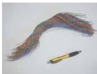
Jim Rist makes inexpensive ties by pulling Cat. 5 wires out of damaged sheathing.
