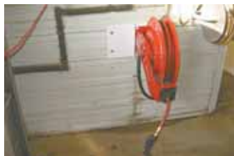
Hinged bracket on retractable hose reel allows the hose to pull out much easier. Reel folds up against shop wall when not in use.
