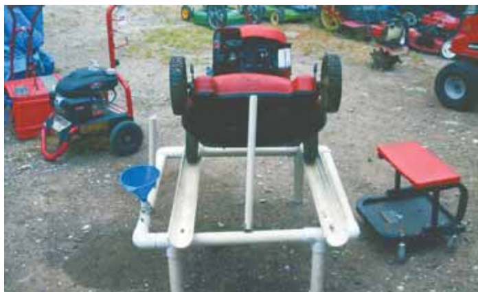
Walk-behind mower rests on a pair of troughs made by cutting a pvc pipe in half. You can prop the mower up from the side or front.
