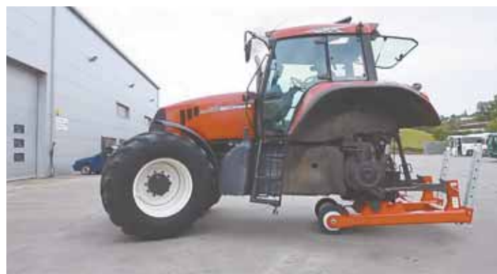
TrakJak slips under tractor’s rear end, attached to the 3-pt. hitch. Tractor hydraulics are used to raise the rear end off the ground.
