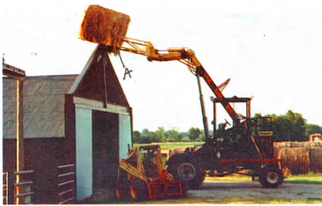
Photo shows size of giant combine loader in relation to New Holland skid steer loader. At point "A", bale is 27 ft. off the ground.
