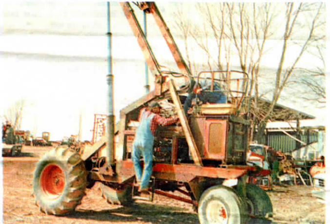
Giant 3-stage telescoping cylinders pivot at bottom. Garton got cylinders off old garbage truck.
