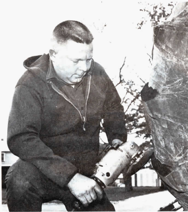
A lot of rubber on this tire, used on a pulling tractor, was removed with a hot knife prior to grinding of the lugs. Operator is simulating lug grinding.
