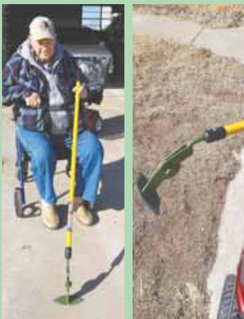
Marion Crum made this adjustable angle hoe by welding 2 sickle blades together and then welding them to a metal bracket. Cutting angle is adjustable using a bolt on the bracket.
