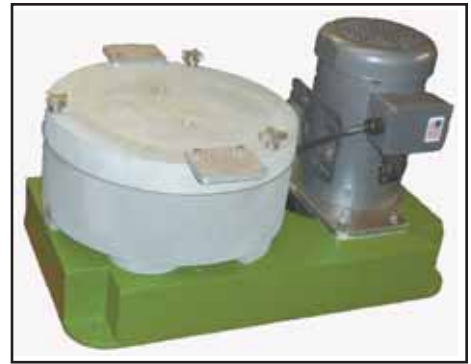
Centrifuge cleans dirty oil so you can use it to safely run diesel engines. It can clean from 10 to 40 gal. per hour.
