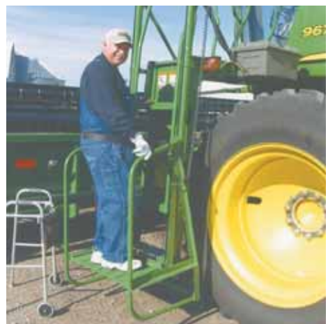
Bolt-on Powerstep lift uses electrical controls at the top and bottom to winch the rider to cab height.
