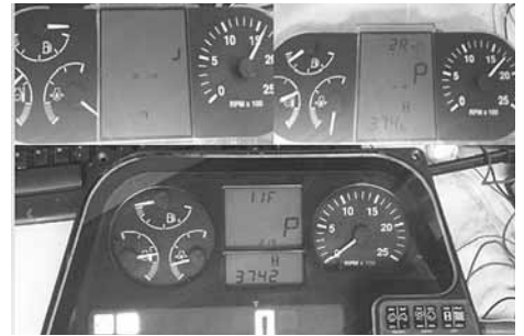
Before (top 2 photos) and after (bottom photo) repair of White 8510 tractor gauges. Gauges would sometimes not work or missing pixels would appear on the display.
