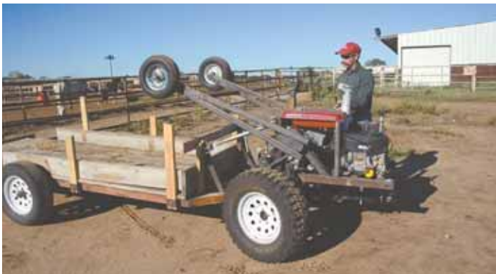
Instead of towing a wagon or other trailing equipment, Mark Lyon's unusual looking single axle tractor actually "self-propels" whatever it's hitched up to.
