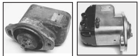
These photos show Calin magnetos before and after they're rebuilt.
