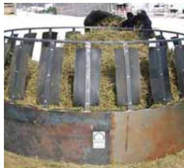
Bale feeder is fitted with 12-in. wide rubber belts spaced 8 in. apart.
