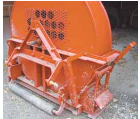
Kurt Cook converted a silage blower into this heavy-duty leaf blower, equipping it with rollers off an old set of reel mowers on front and back so it rolls over uneven ground.
