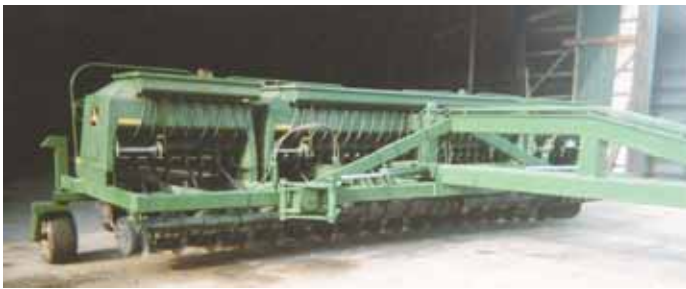
Rusty Inskeep and his nephew Paul rebuilt two 15-ft. Deere 1590 no-till grain drills into a single machine equipped with 6-ft. folding wings.
