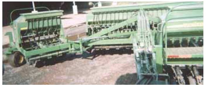
Wings were made by cutting apart one of the drills and removing the rear frame and wheels. Wings pivot 180 degrees forward for road travel.
