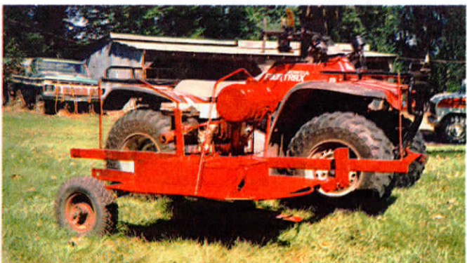
One side of deck is supported by a 6-in. wheel. Other side bolts onto brackets welded to front and rear of ATV.
