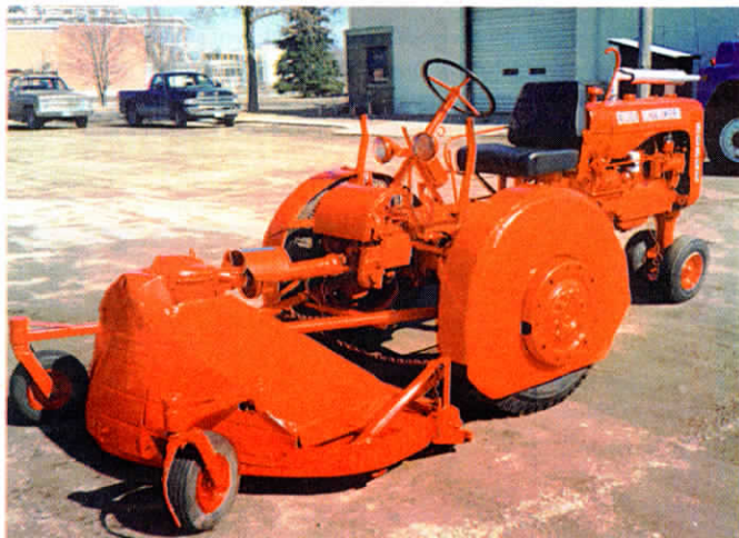
Thor reversed the controls on his Allis Chalmers CA tractor and built mower deck that's pto-driven by an automotive rear end mounted vertically above deck.
