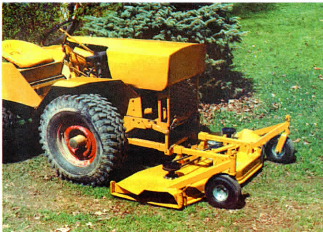
Mower deck's three 22-in. blades cut about 5 1/2 ft. wide and are belt-driven off engine.
