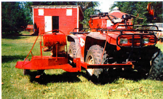
Side-mount mower is powered by an 8 hp Briggs & Stratton gas engine that belt-drives a single 26-in. blade. It mounts on Malone's Honda 350 4-WD ATV.
