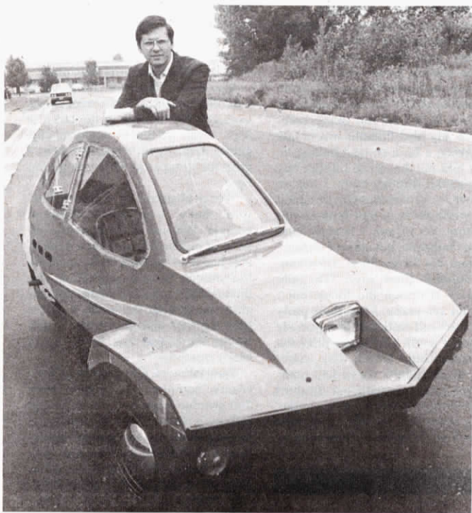
Three wheeler is powered by a 9.6 hp. diesel engine.
