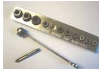
Make Sense Tap Adapters fit over the head of a tap and can then be turned with conventional wrenches or sockets.
