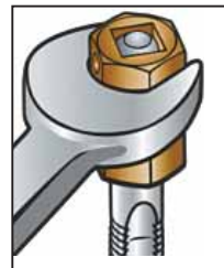
Make Sense Tap Adapters fit over the head of a tap and can then be turned with conventional wrenches or sockets.
