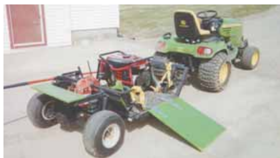
Tom Haney turned an old golf cart into this portable power tool cart. A ramp makes it easy to load his emergency generator.
