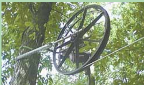
Wood carrier retracts like a pulley-equipped clothes line, using an electric drill. Wheelchair wheels serve as pulleys at either end of zip line.
