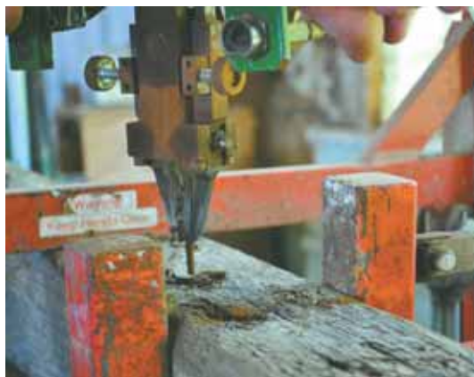
Buried nails can really lower the value of old barn wood, but pulling them out by hand is slow work. To make the job go faster Dan Yoder had a local machinist build this power denailer.
