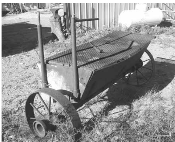
Made out of an old loader bucket, this portable barbecue grill rides on steel wheels and has a tongue on front for pulling behind an ATV.
