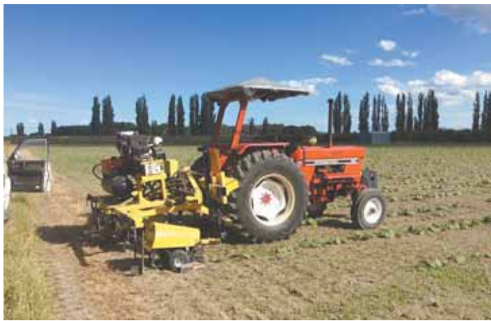
Andy Lysaght's inter-plant weeder eliminates hand weeding in high-value, precision-placed crops. It requires no computers, circuit boards or programming.
