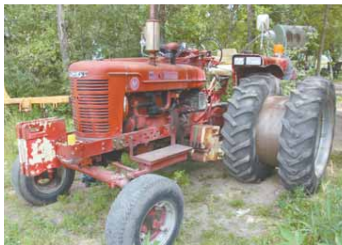
Mike Bauer’s Farmall “M” has plenty of unusual features, including 38-in. rear wheels with matching solid rim wide-band duals.
