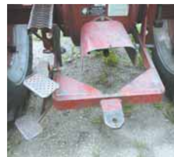
Right side of engine is fitted with a conglomeration of hydraulic pumps, belts, hoses and reservoirs (left). On back, Bauer rebuilt the hitch into a reinforced 3-pt. connection.
